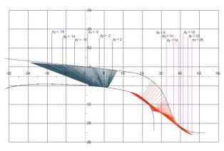
Simulation of wheel-rail contact points using GENSYS
