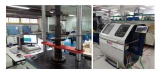
Static press (Ibertest) and wheel tracking (Hamburg Wheel tracker)
