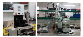
Colloidal mill to produce bituminous emulsions and rotary evaporators
