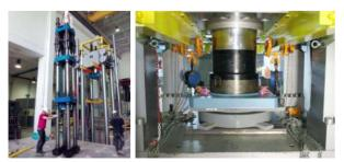
Fatigue tests of prestressed systems and tests of support devices of confined neoprene (High capacity press MTS-15MN)
