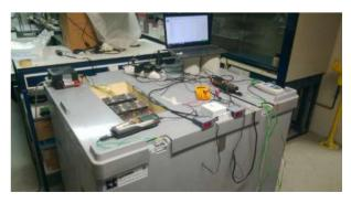
Hot-Box: Measurement of the thermal properties of materials and elements
