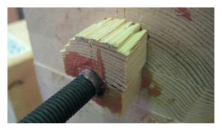
Systems to improve the anchor of steel bars glued to wood
