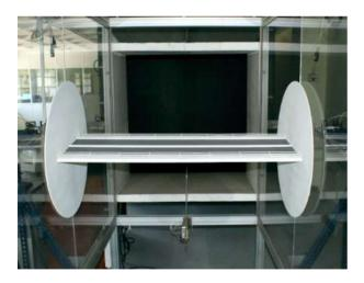
Aeroelastic test on a section of a bridge deck
