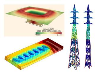
Surface passing potential originated by the ground of a buried substation, pressure in a fracked shale gas well, and optimization of a high-tension tower
