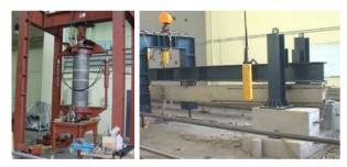
Tests of graphite electrodes and prestressed reinforcement anchorage
