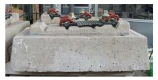
Prefabricated block for mounting the fastening of the rail in the slab track prototype
