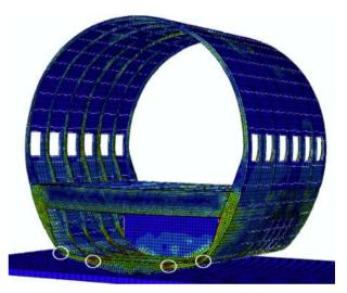
Map of the deformations of the fuselage structure of a Boeing 737
