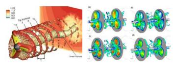
Horizontal marine turbine to generate energy and dynamics of an oscillatory bioreactor with three holes for biofuel production
