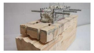
Connectors of composite section Glulam-Concrete and Glulam+CLT
