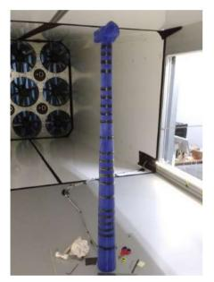
Test in a boundary layer wind tunnel with vertical junctions of prestressed concrete aerogenerator towers
