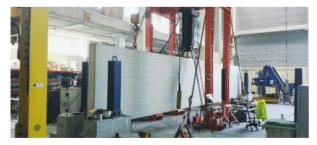
Shear test of a concrete beam of 2 m height (European Record)
