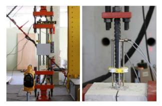
Reinforcement lap and bar anchorage tests
