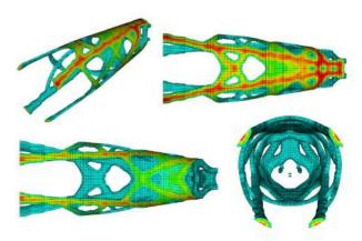
Models to optimize the fuselage rear section of a plane
