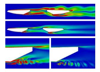
Vorticity maps in sections of long-span multibox bridges simulated with CFD
